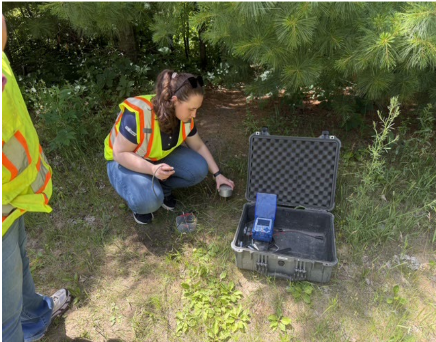
Facing west near MP 2.79, view of seismograph staged near the exit side of HDD P4-5
